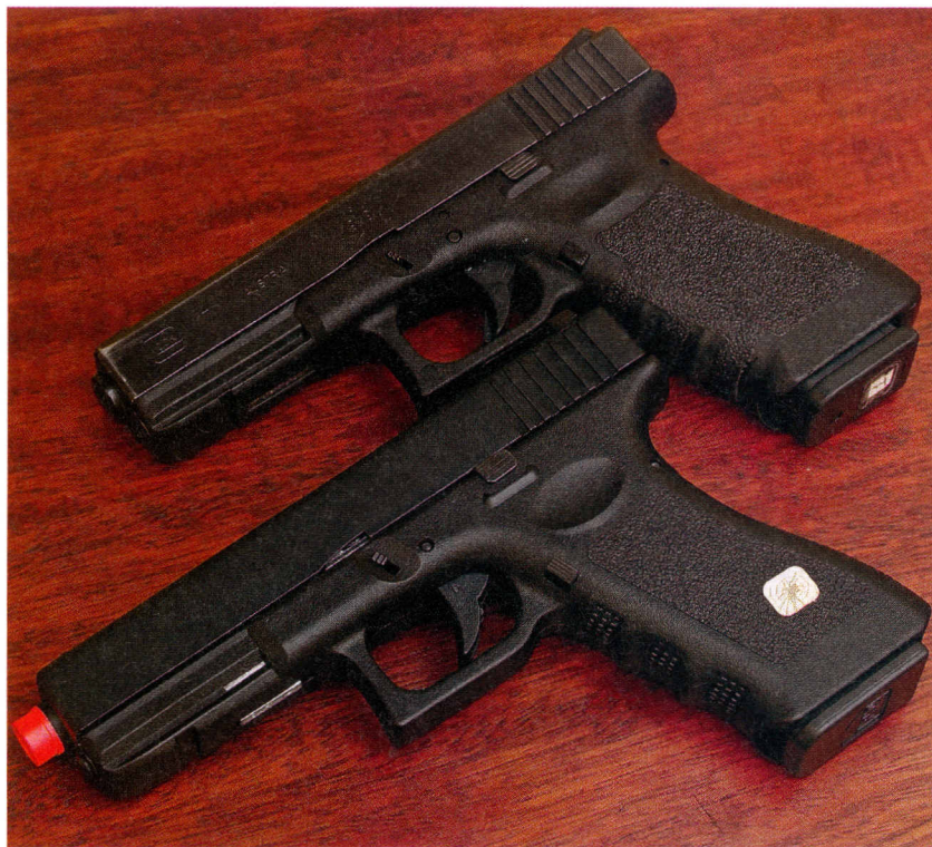
The HFC Airsoft at bottom is based on the Glock 17. Note that the HFC does not feature the actual Glock's trigger safety system.
